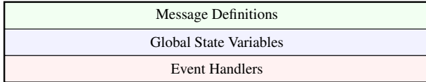
Figure 2: Schematic overview of PSF that consists of: (1) protocol message formats, (2) global variables used by event handlers; and (3) event handling functions.
